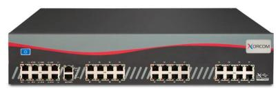
PRI/R2/CAS ISDN E1/T1 port. The XR2000 supports up to 160 PSTN / Analog phones ports with external Astribank units, up to 200 users and up to 85 concurrent calls.
